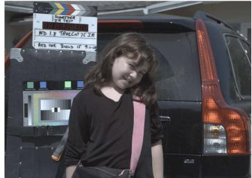
Captured with RED One Camera, Build 15, Angenieux Optimo 17-80, F5.6, with ND 1.8 - No IR Filter
